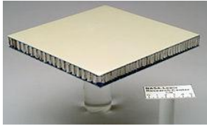
Composite sandwich structure panel used for testing at NASA
